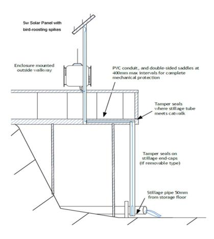
Figure 2— Installation Type 2 storage meter - elevated platform with a submersible pressure sensor for storage metering.
